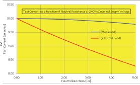
Voltage from the Phase-Earth Voltage measured across the ModieLoad as outlined in Step (10) of the AS4741 Testing Operating Instructions.
